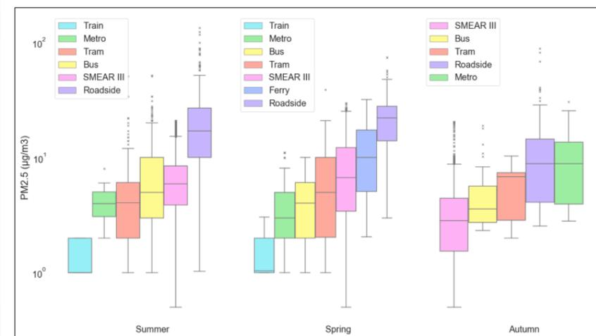
Fig. 4. The PM<sub>2.5</sub> level in different transportation systems during our experiments.
