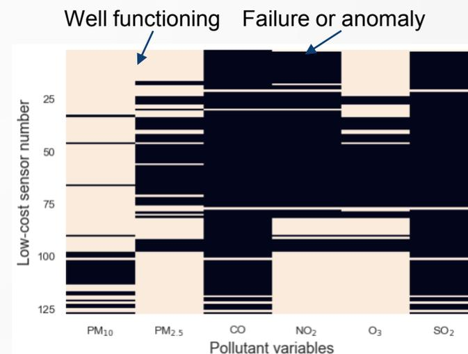
Individual analysis: sensors failure and anomaly
